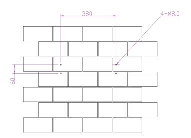
Figure 3.4 Drill holes dimensions of H2 inverter
