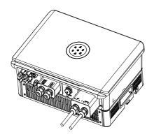
Figure4.7 Positive and negative connectors
