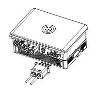
3.Secure all parts of the grid and backup connector tightly.
