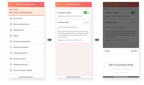
5.4.2 Working modes introduction **Self-consumption Mode:** When the solar is sufficient, electricity generated by photovoltaic system will be supplied to load first, the surplus energy will be stored in battery, then the excess electricity will be exported to the grid. When the solar is insufficient, the battery will release electricity to supply load.
