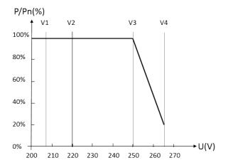
Figure 5.3 Curve for a Volt-Watt response mode (AS4777 Series)
