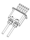
2.Fix the cables according to conductor marks of L, N and PE.
