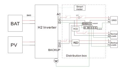
The system connection for grid system without special requirements is as below.
