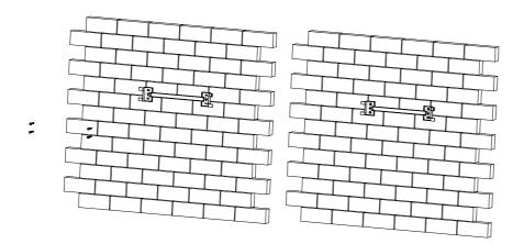
Figure 3.5 Mount the Rear Panel of H2 inverterr
